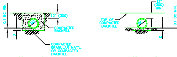
GRANULAR FOUNDATION TRENCH
